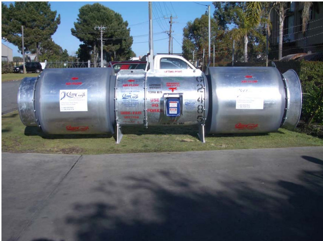
Figure 1 – CC925 1x45kW Single-Stage Axial Fan c/w Silencers, Inlet Cone and Duct Adapter
