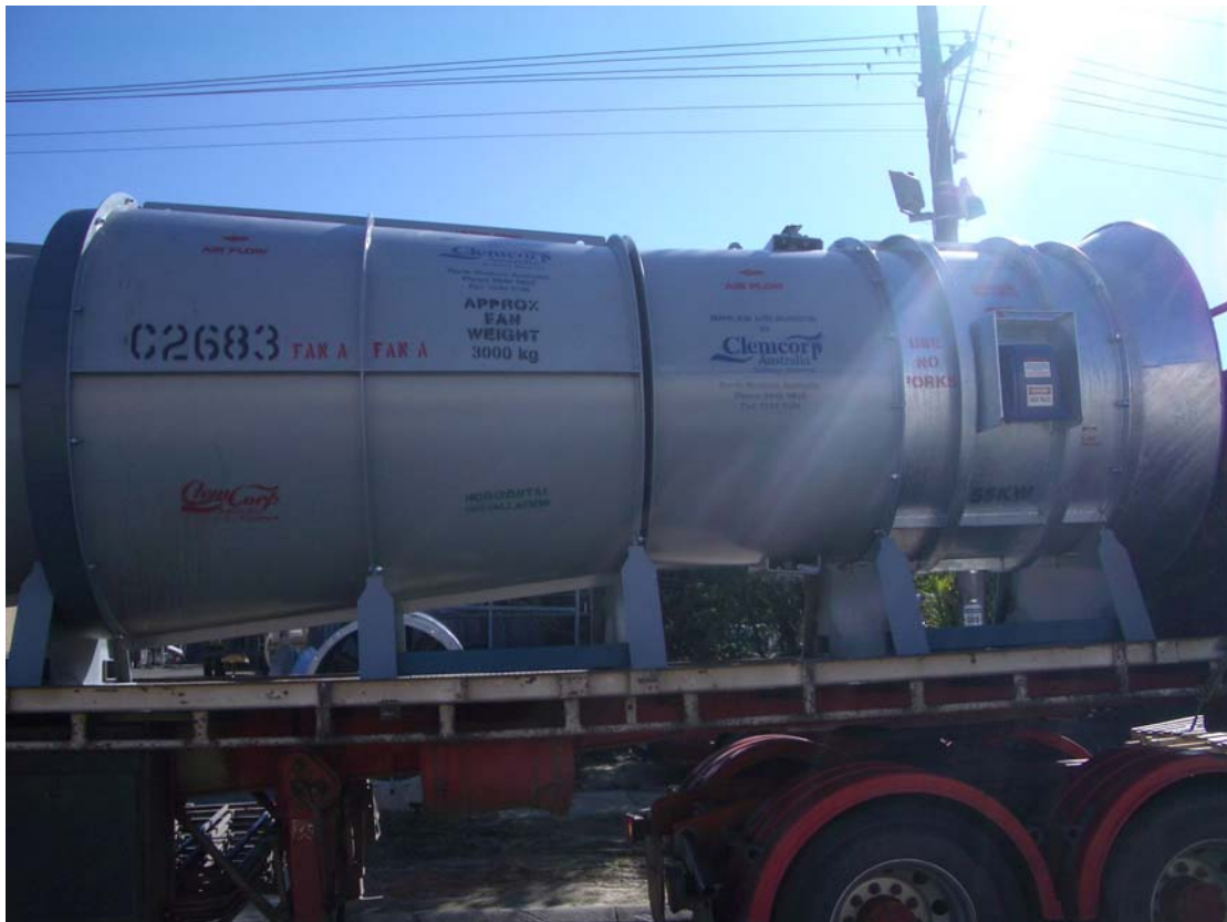
Figure 1 - CC1524 1x55kW Single-Stage Axial Fan c/w Diffuser, Extended Feet, Inlet Cone and Self-Closing Doors
