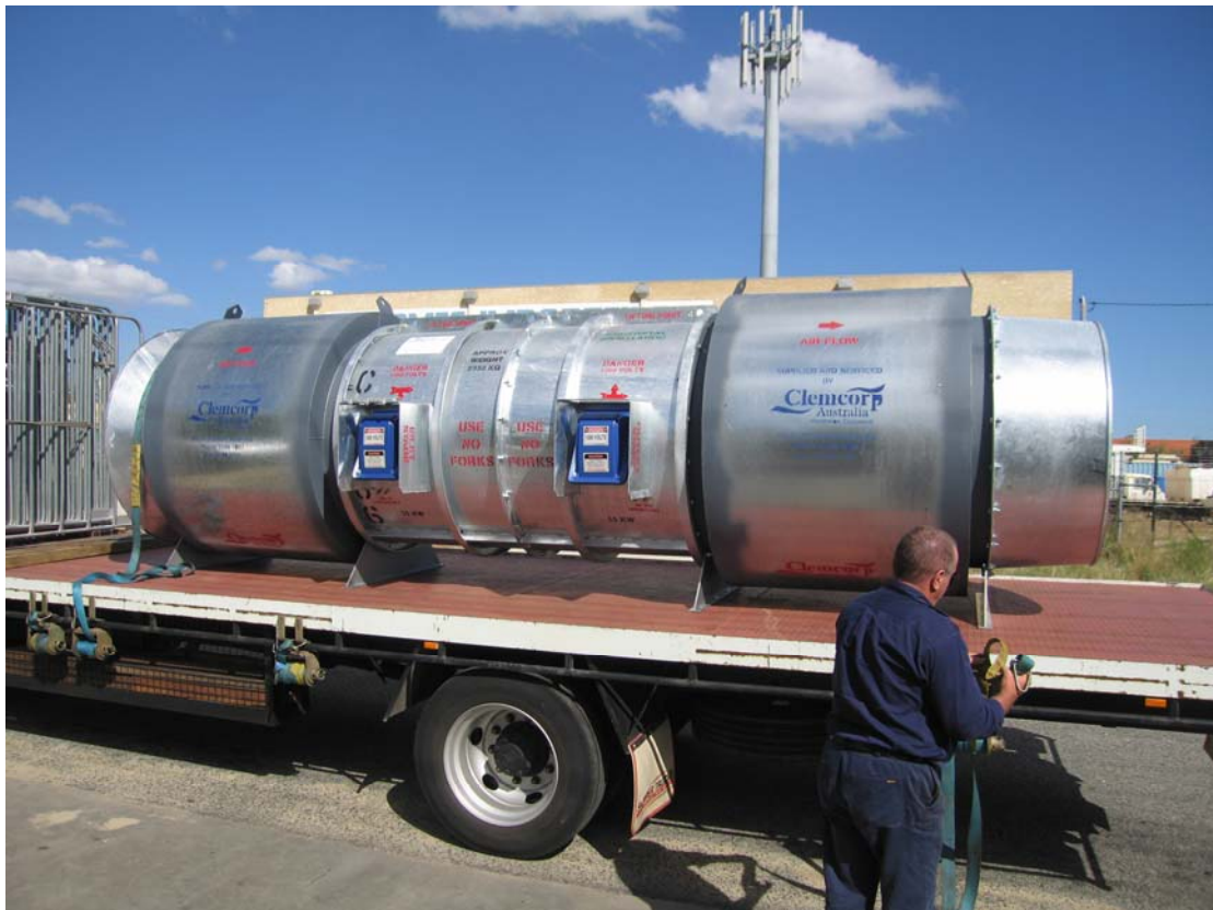
Figure 1 - CC1254 Mk3 2x55kW Contra-Rotating Axial Fan c/w Silencers, Inlet Cone and Duct Adapter
