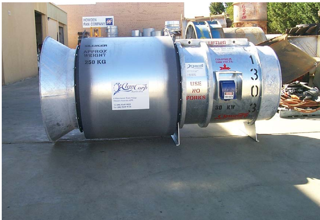
Figure 1 - CC1070 1x30kW Single-Stage Axial Fan c/w Silencer, Inlet Cone and Duct Adapter
